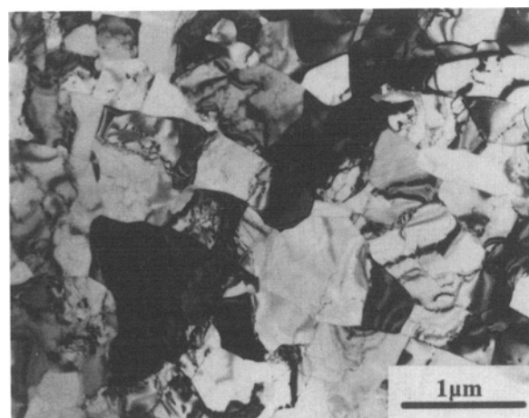
Fig. 12 TEM image of sample VI rolled at a reduction in thickness of 95%
